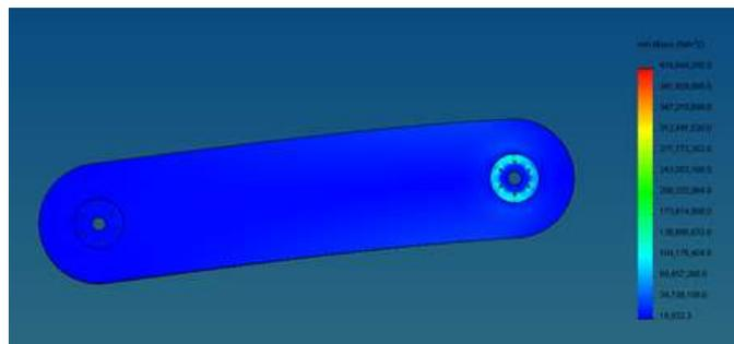
Fig. 4. Stress on Arm Due to Load
