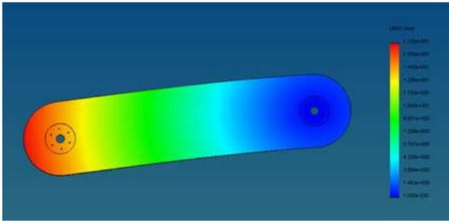
Fig. 5. Displacement of Arm Under Load (Exaggerated)
