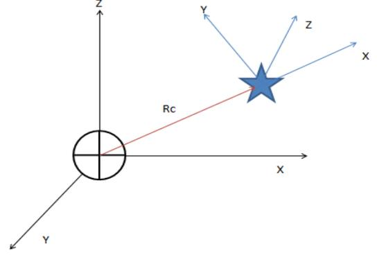
Fig. 1: The spacecraft in the LVLH frame.
