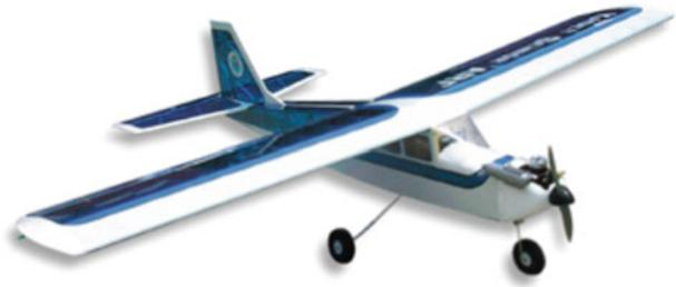
The sensors used were a GPS module with a LEA-5H chip with an accuracy of 2.5 m CEP. The IMU has an orientation accuracy of  $\pm 2.0^\circ$ . For data communication the Maxstream 2.4 GHz modem was used, with a range of 10 miles. A camera and a separate modem were used for video transmission. Figure 23 shows the UAV used for experimental verification, while Table 4 gives its specifications.
