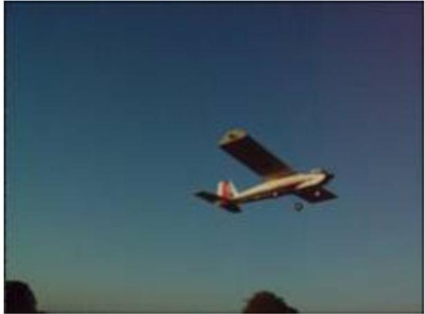
The first flights were conducted to test the communication between the UAV and the ground station and to gather data from the different sensors. For these tests the airplane was controlled by remote control not the autopilot.
