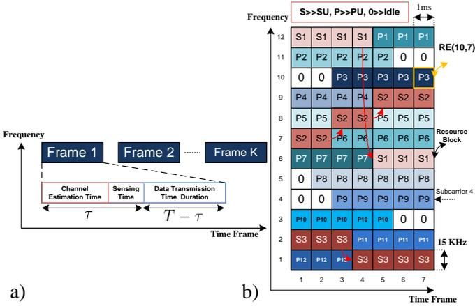
Fig. 2. a)Timing Model, b)Resource Block & Dynamic Resource Management
