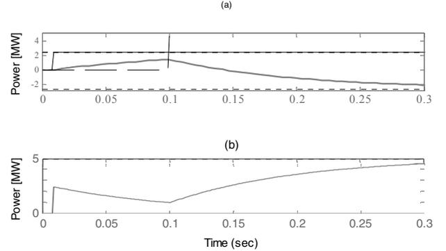
Figure 3: (a) Response of power consumed by station (gray) in response to step changes in EV charging power (solid) and grid support (dashed) according to equation (21) and (b) response of power supplied by battery.
