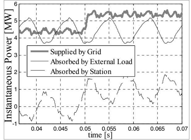
Figure 8: Instantaneous power supplied by the grid, absorbed by the external load, and absorbed by the charging station during simulation.
