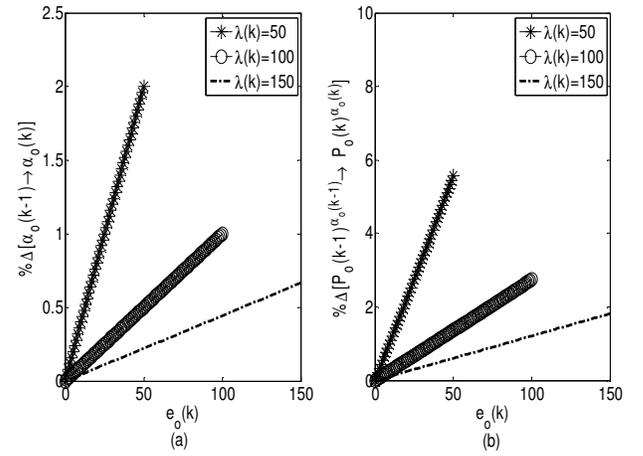
Fig. 6. For  $\lambda(k) = (50, 100, 150)$  comparison of (a) the percentage of change in alpha from  $(k - 1)$  to  $(k)$  vs. the magnitude of  $e_o(k)$  and (b) the percentage of change in transmit power from  $(k - 1)$  to  $(k)$  vs. the magnitude of  $e_o(k)$ .
