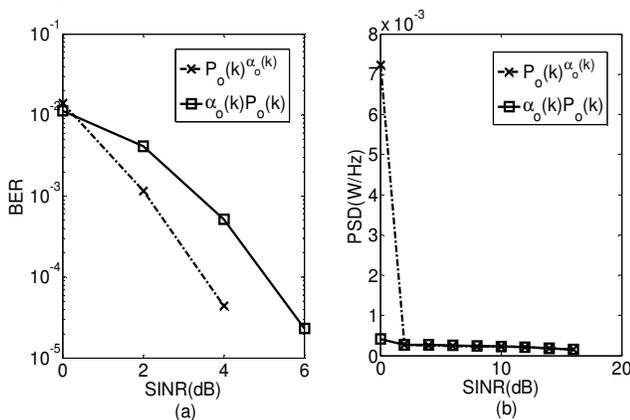
Fig. 7. Comparison of  $\alpha_o(k)$  and  $\alpha_u(k)$  used in BER-TPC as exponent and scalar for SINR vs. a) BER and b) PSD(W/Hz).
