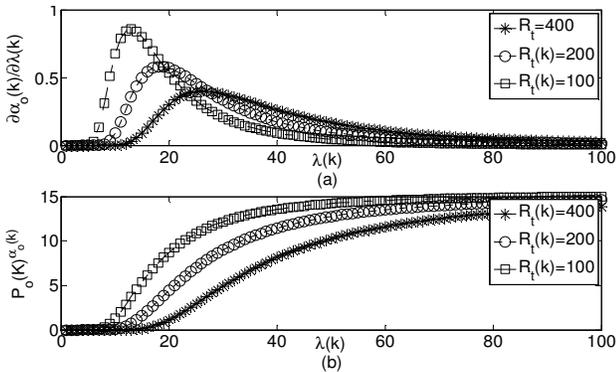
Fig. 5. For  $R_t(k) = 400, 200, 100$  (a)  $\lambda(k)$  vs.  $\frac{\partial \alpha_o(k)}{\partial \lambda(k)}$  and (b)  $\lambda(k)$  vs transmit signal power  $[P_o(k)^{\alpha_o(k)}]$ .
