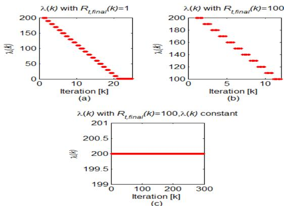
Fig. 3. Approximator inputs to test critical points of  $\lambda(k)$ : (a) tracking  $R_t(k)$  as it decrements from a value of 200 to 1, (b) tracking  $R_t(k)$  from 200 to 100, (c) not tracking  $R_t(k)$   $\lambda(k)$  is constant.
