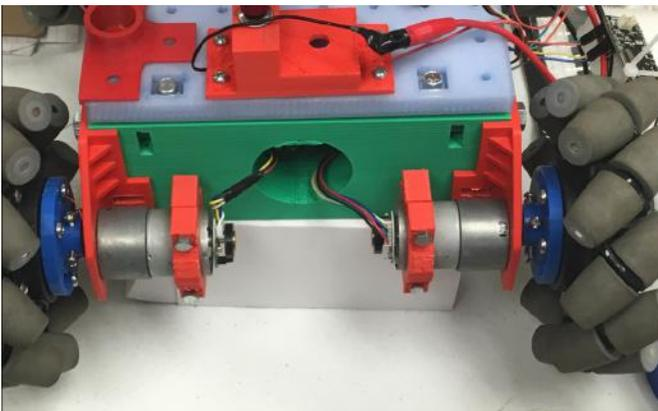
Fig. 3: Pololu DC motor with wheel encoders mounted to chassis
