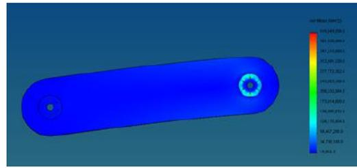
Fig. 6: Stress on arm due to load
