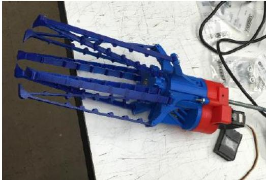
Fig. 9: Underactuated gripper in an almost closed state
