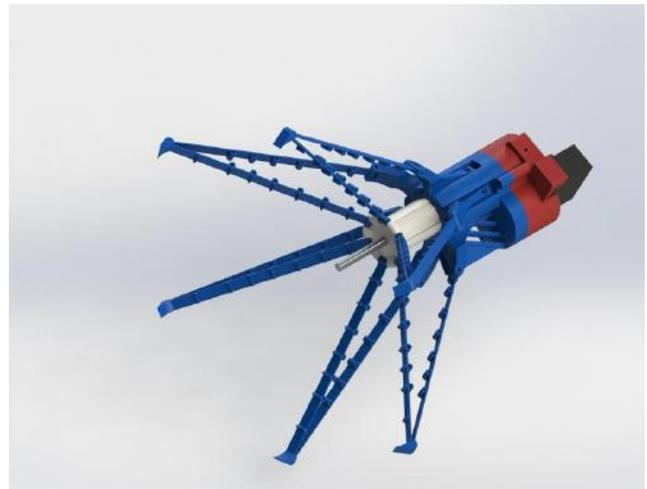
Fig. 10: SolidWorks render of underactuated gripper in an open state
