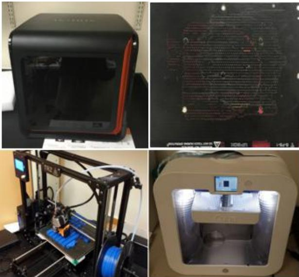
Fig. 1: UPBOX (Top Left), UPBOX Build Plate (Top Right), Lulzbot Taz 4 (Bottom Left) and Cube 3 (Bottom Right)
