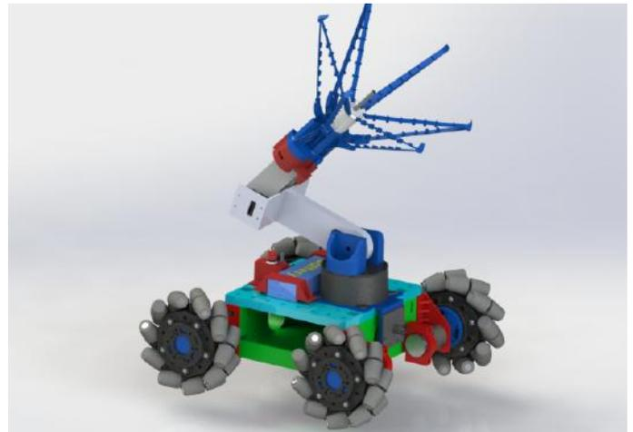
Fig. 11: SolidWorks render of underactuated gripper with new manipulator arm
