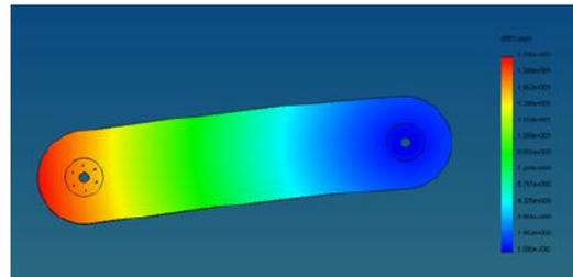
Fig. 7: Displacement of arm under exaggerated load
