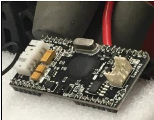
Fig. 13: EasyVR3 module for voice recognition
