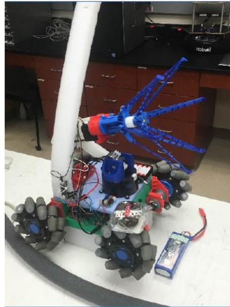
Fig. 14: Final voice controlled robot
