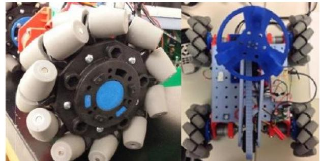
Fig. 2: Mecanum wheel (left) and positioning of wheels (right)
