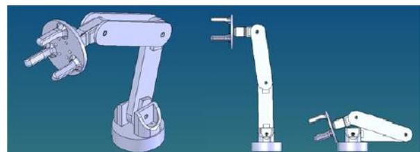
Fig. 5: Design of valve turning manipulator arm
