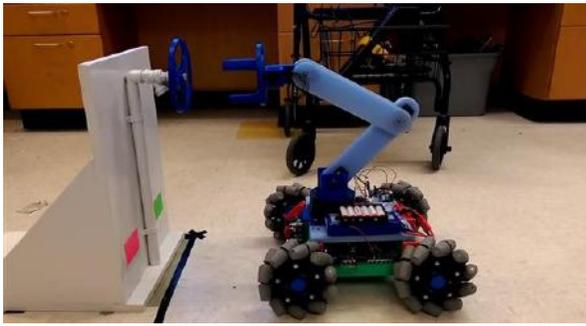
Fig. 8: Final design of valve turning robot next to valve
