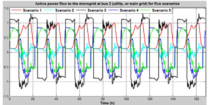
Figure 6 Power Exchange with the Utility or Main Grid; Five scenarios
