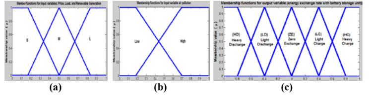
**Figure 3 Fuzzy Membership functions for input and output variables of the Fuzzy Controller; (a) price, load and generation (b) air pollution (c) output**
