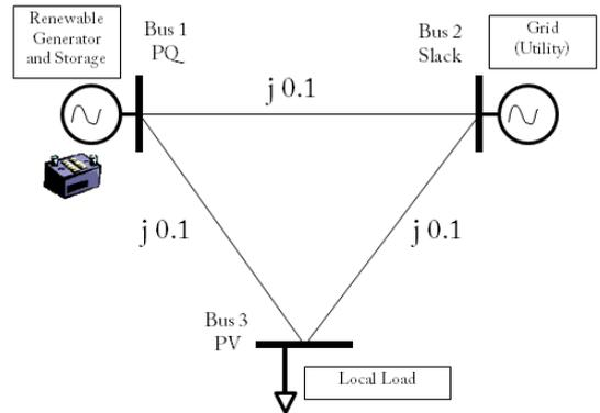
Figure 2 Three Bus Model of microgrid
