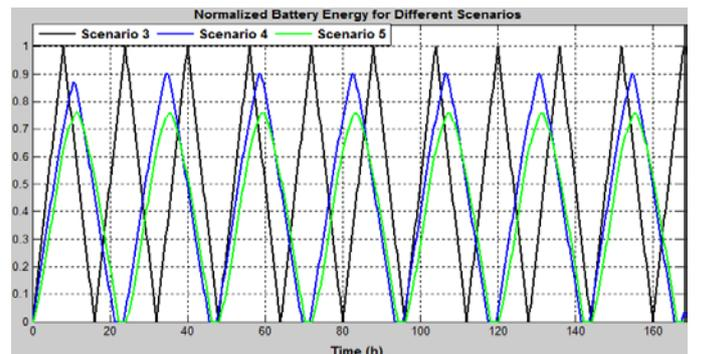
Figure 8 Normalized Battery Unit's Energy over a week; Five Scenarios
