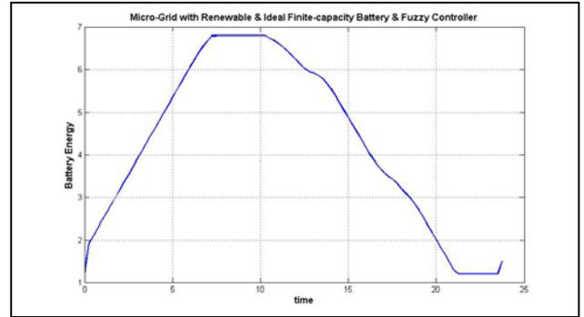
Figure 11 Measure of Energy stored in Battery; scenario 3
