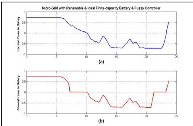
Figure 10 Output of the Fuzzy Controller; scenario 3; (a) Theoretically allocated (b) Practically feasible
