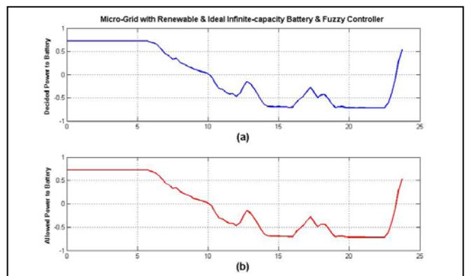
Figure 8 Output of the Fuzzy Controller, i.e. measure of the amount of power given to/taken from storage unit; scenario 2; (a) Theoretically allocated (b) Practically feasible
