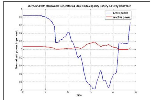
Figure 12 Power Flow of Bus 2 connected to Utility; scenario 3
