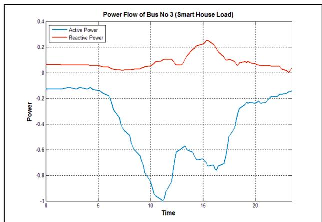
**Figure 10 The Power Flow of Bus 3 including Load (Smart House) in a typical day for each 15min period with storage on bus 2**
