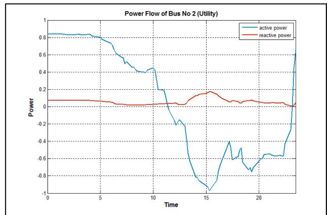
**Figure 9 The Power Flow of Bus 2 connected to utility in a typical day for each 15min period with the Storage on bus 2**
