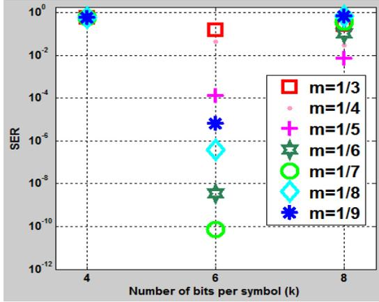
Fig. 2. SER for  $2^k$ -QAM channels vs. K; ac electrical power at -5dBm
