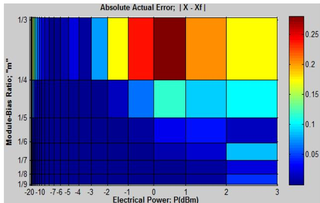
Fig. 6. Actual absolute error between the estimated SER and the actual SER
