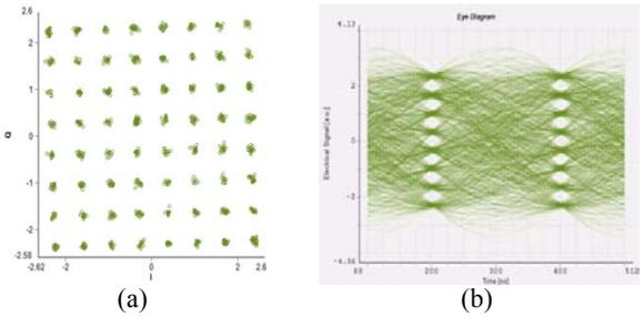
Fig. 4. Received and detected signal for 64-QAM channel with carrier frequency= 397.25 (MHz); (a) Constellation (b) Eye Diagram
