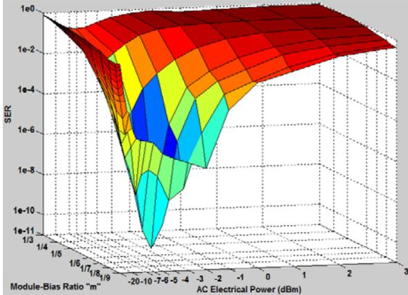
Fig. 3. SER vs. “m” and ac electrical power for received 64-QAM channel with carrier frequency= 397.25 (MHz)
