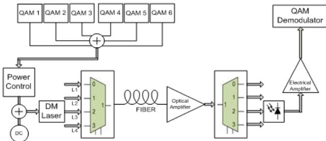
Fig. 1. System of RoF multiplexed on 4-WDM
