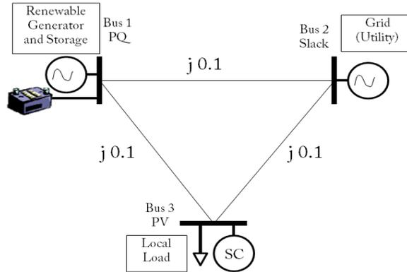
Figure 2 Three Bus Micro-grid Model
