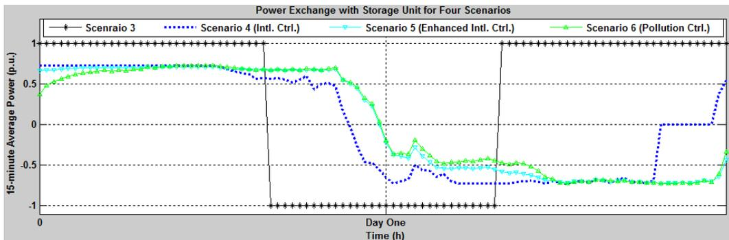
Figure 10 Normalized Battery Power Flow; First Day; Four Scenarios
