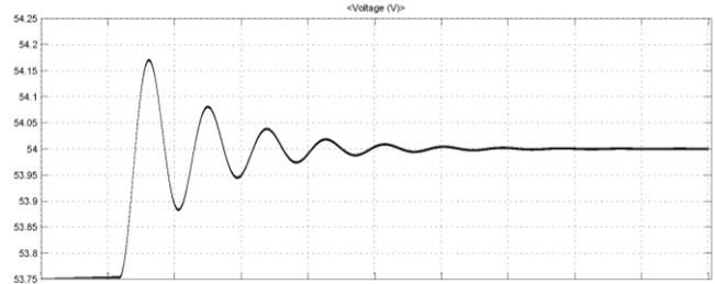
Fig. 7. output voltage transient response with PI controller
