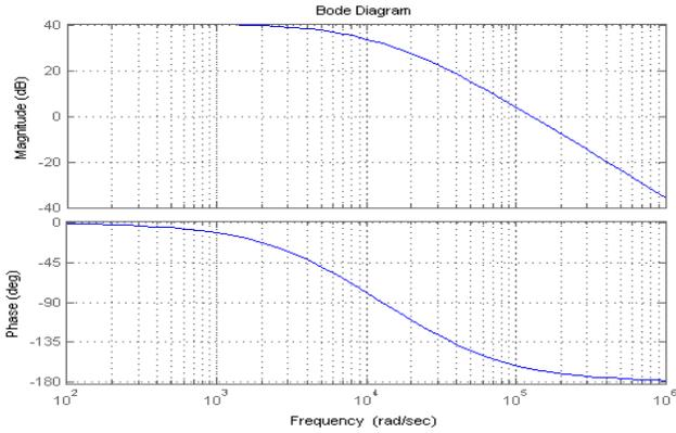
Fig. 6. converter control-to-output transfer function
