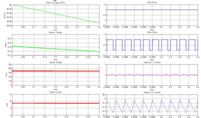
Fig. 11. Battery Boost Mode Results.
