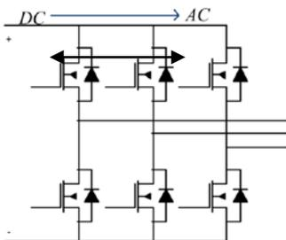
Fig. 4. A three phase full bridge inverter can act as a diode bridge rectifier in reverse when no signals are sent to the gates.
