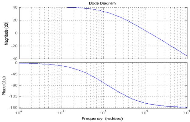
Fig. 6. converter control-to-output transfer function
