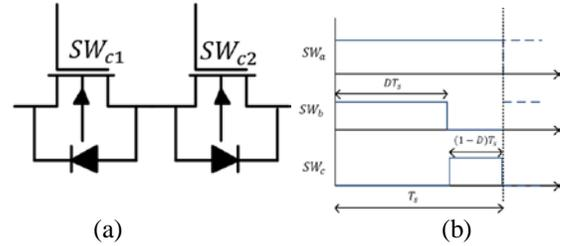
Fig.13. (a) Four Quadrant Bi-Directional Switch. (b)The basic order of switching operation to charge the battery from energy of the PV source and the rectified grid voltage simultaneously.
