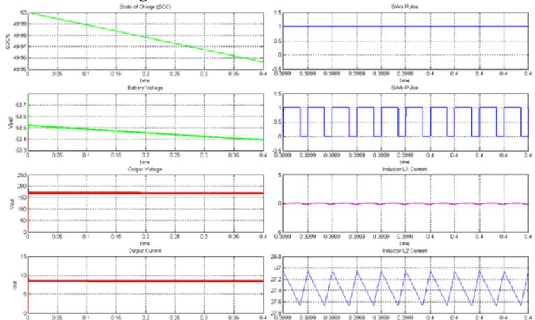
Fig. 11. Battery Boost Mode Results.
