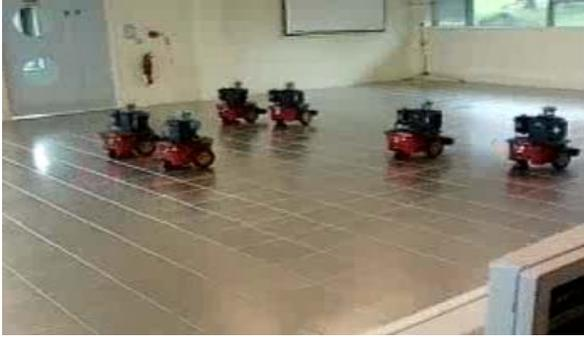
Fig. 2. A mobile robot controls a group of robots using the developed multi-robot network
