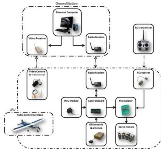
Figure 8. Hardware implementation of the testbed
