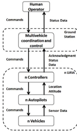
Figure 1. Architecture of the system
