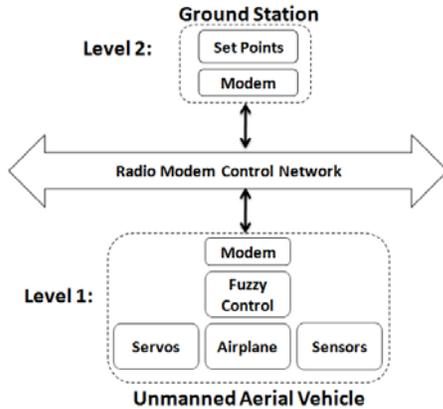
Figure 3. Hierarchical structure of NCS for one UAV
