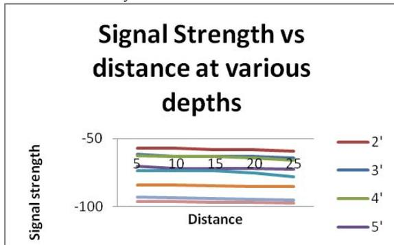
Figure 10. Xbee Pro module signal strength underwater
