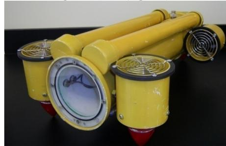
**Figure 7 Robot chassis and thrusters with floatation units**
