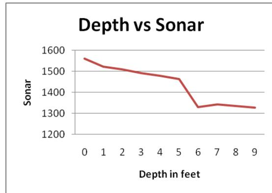
Figure 11 Sonar reading vs. measured depth
