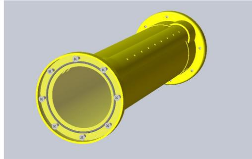
**Figure 6 Robot body with sealed ends and Ballast strip**
