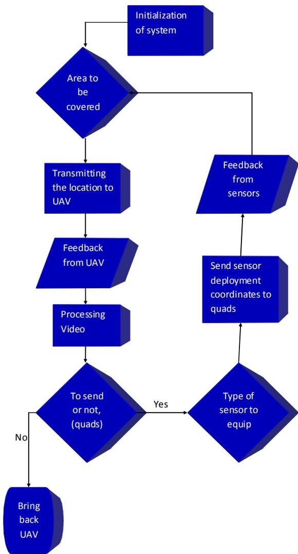
Figure 4. Software algorithm flowchart diagram.
