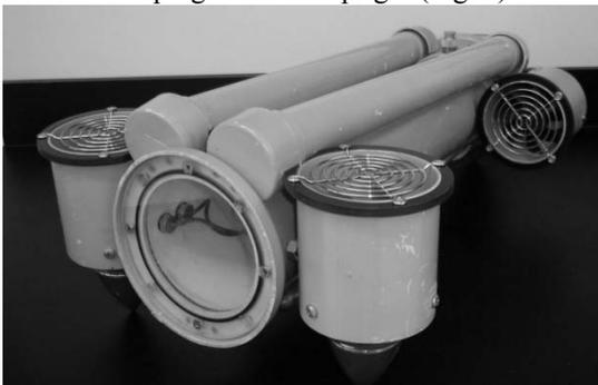
Fig. 3 Robot chassis and thrusters with floatation units
