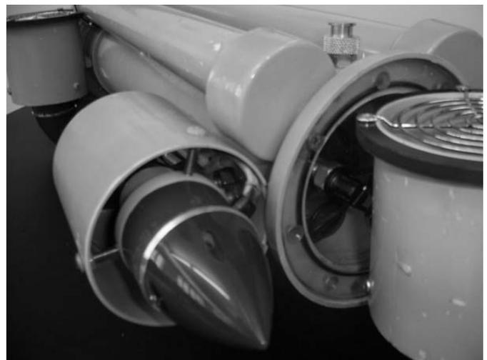
Fig. 5 Thruster showing bilge pump
