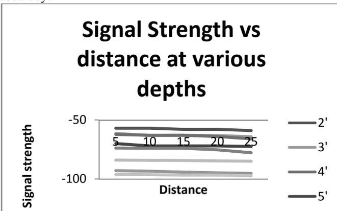
Fig. 9 Xbee Pro module signal strength underwater
